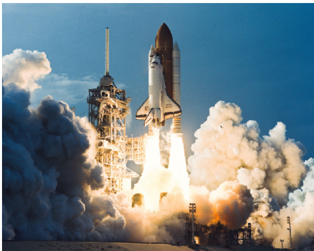
Figure 3.7 Demonstrating Newton's Third Law. The U.S. Space Shuttle (here launching Discovery ), powered by three fuel engines burning liquid oxygen and liquid hydrogen, with two solid fuel boosters, demonstrates Newton's third law. (credit: modification of work by NASA)
